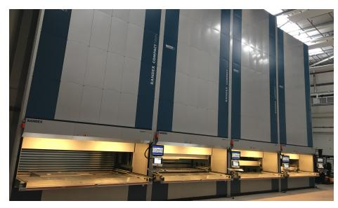
'Compact' vertical storage lifts save up to 90% of floor space compared to standard shelving and pallet racking. They can manage loads of up to 100 metric tonnes and enable warehouse operatives to complete up to four times more picks than in a traditional warehouse, with goods automatically presented to the picker.
