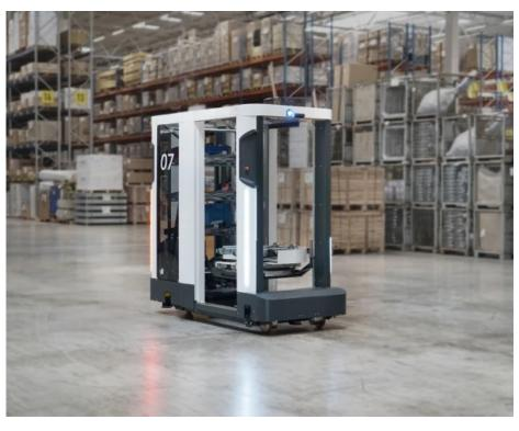
material from the automated warehouse to the assembly line. There, the robot transfers the KLT to flow racks. At the same time, the robot also handles the return transport of empties. The VDA KLT can weigh up to 20 kilograms and have a footprint of up to 600 x 400 millimeters. Cameras and sensors allow safe operation alongside humans — the cameras are also used to identify the correct pick-up and delivery shelves via Data Matrix Codes."
